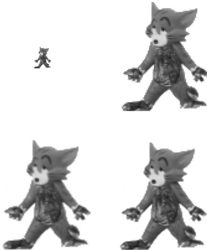
Fig. 6. Image interpolation methods: the original image (top left) was enlarged five times using three different interpolation techniques—nearest neighbor (top right), bilinear (bottom left), and bicubic (bottom right).
